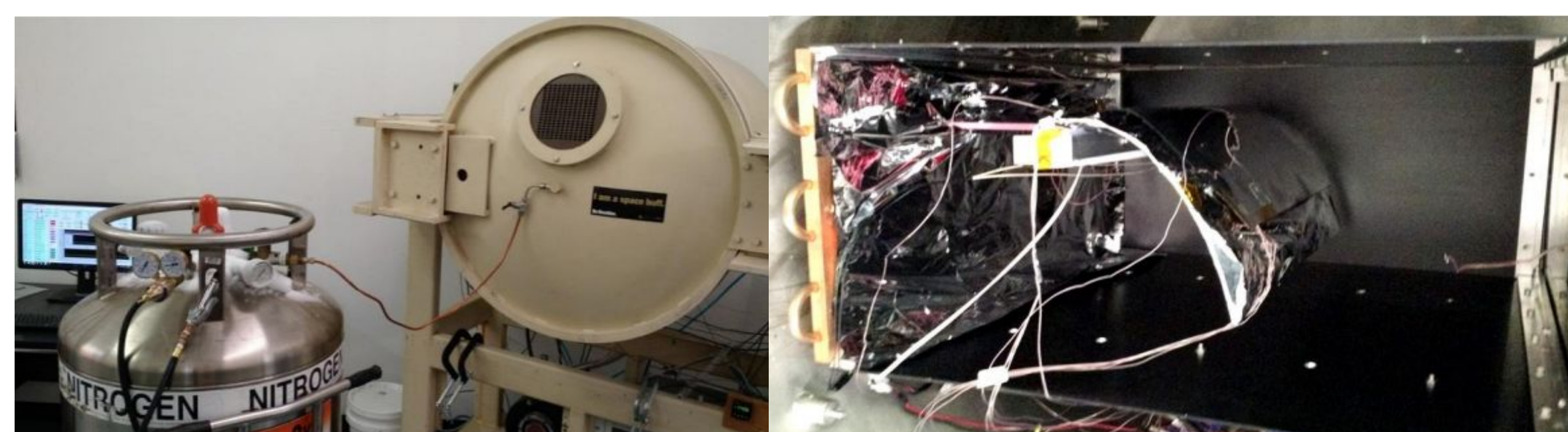
Backfilling the test chamber with cold GN2
