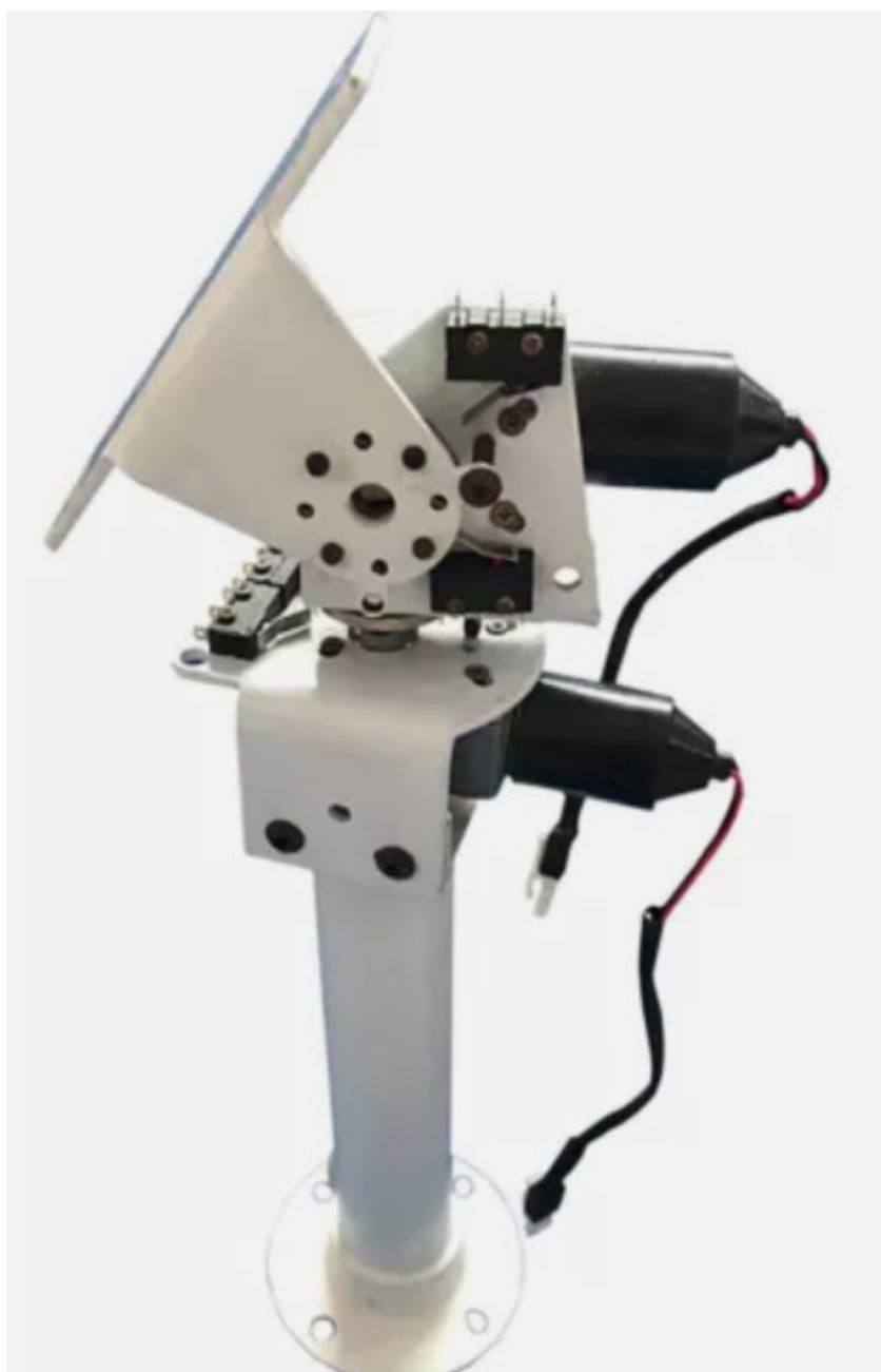
Heliostat Control Arm
