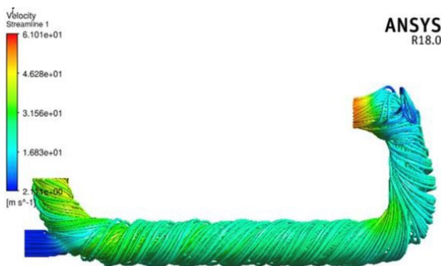
Figure 4: Ansys Simulation of Flow Swirling in Pipe
