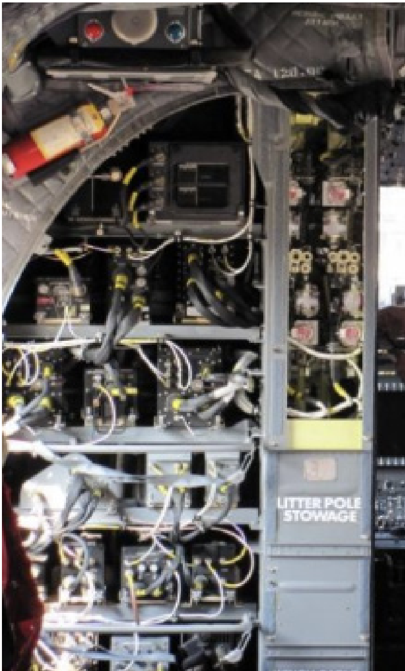
Current Avionics Rack in the Chinook CH-47
