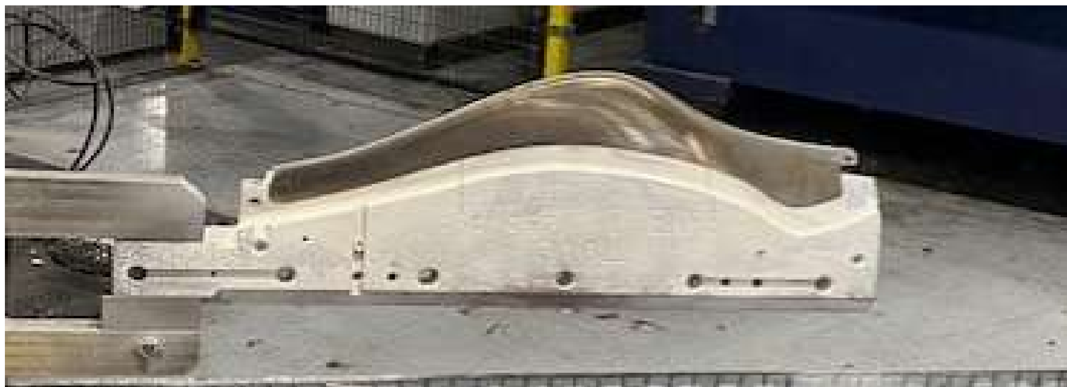
Leading Edge Blade on the Mandrel
