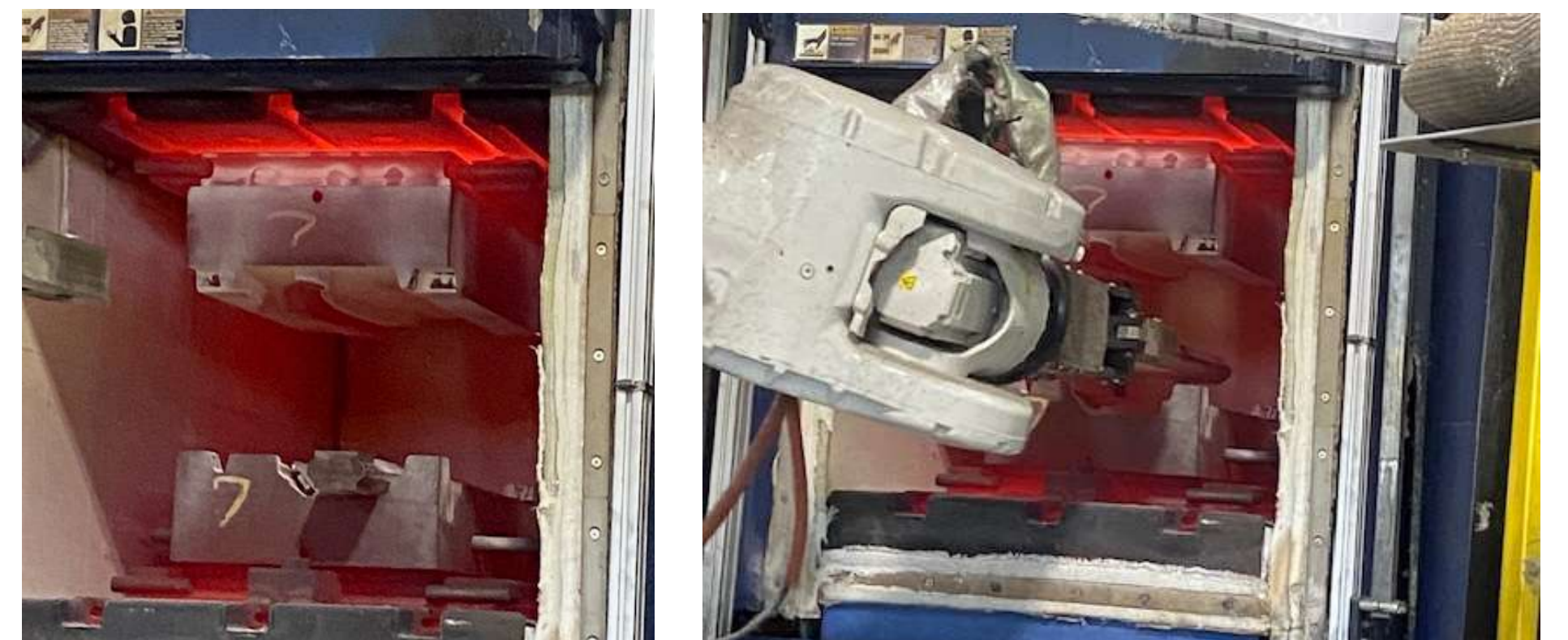
Heated Power Form Press and Forming Process
